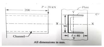
4. A rectangular steel plate is welded as a cantilever to a vertical column and supported a single concentrated load P, as shown in figure below. Determine the weld size if shear stress is not exceed 140 MPa.
