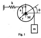
11. A vibrating system is defined by the following parameters: m= 3 kg, k= 100 N/m, C=3 N-sec/m Determine: a) damping factor, b) the natural frequency of damped vibration, c) Logarithmic decrement, d) the ratio of two consecutive amplitudes and e) The number of cycles after which the original amplitude is reduced to 20 percent.
