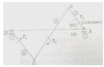
22. Find the torque required to be applied to link AB of the linkage shown in figure to maintain static equilibrium. The force F is perpendicular to link CD acting at E. The dimensions of the links are in mm.
